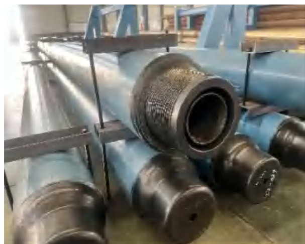
Physical diagram of double-walled drill pipe
